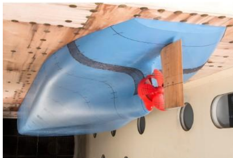
FIGURE 2-7 FULL SHIP MODEL IN CAVITATION TANK
